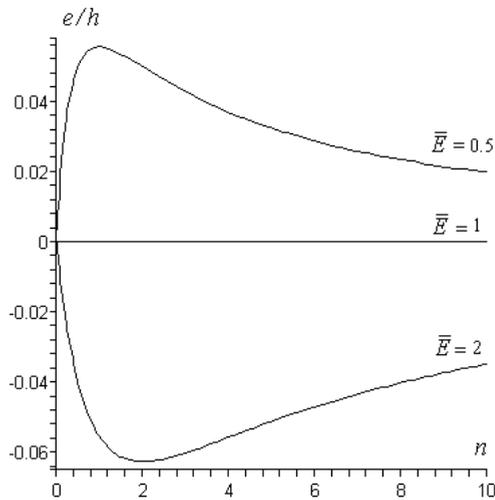
Fig. 5 Dimensionless depth of N.A. for rectangular FGB
