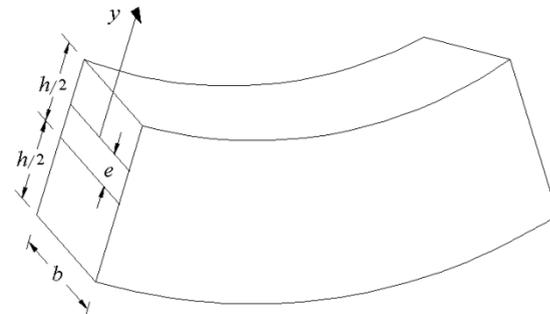
Fig. 1 Origin of y-coordinate for rectangular section
