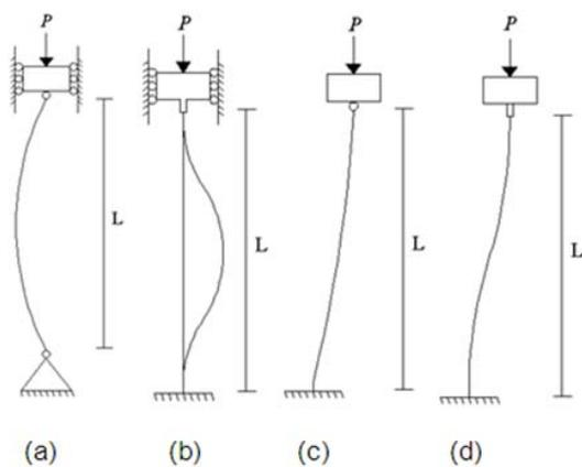
Fig. 2 Buckling of FGB with various boundary conditions
