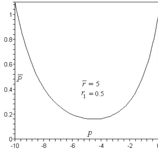
Fig. 7 Local minimum for  $\bar{P}$  in annular FGB
