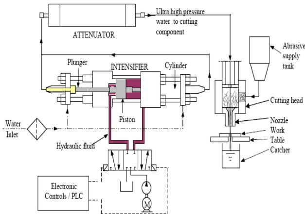
Fig. 1 A setup of an AWJ cutting machine [1]
