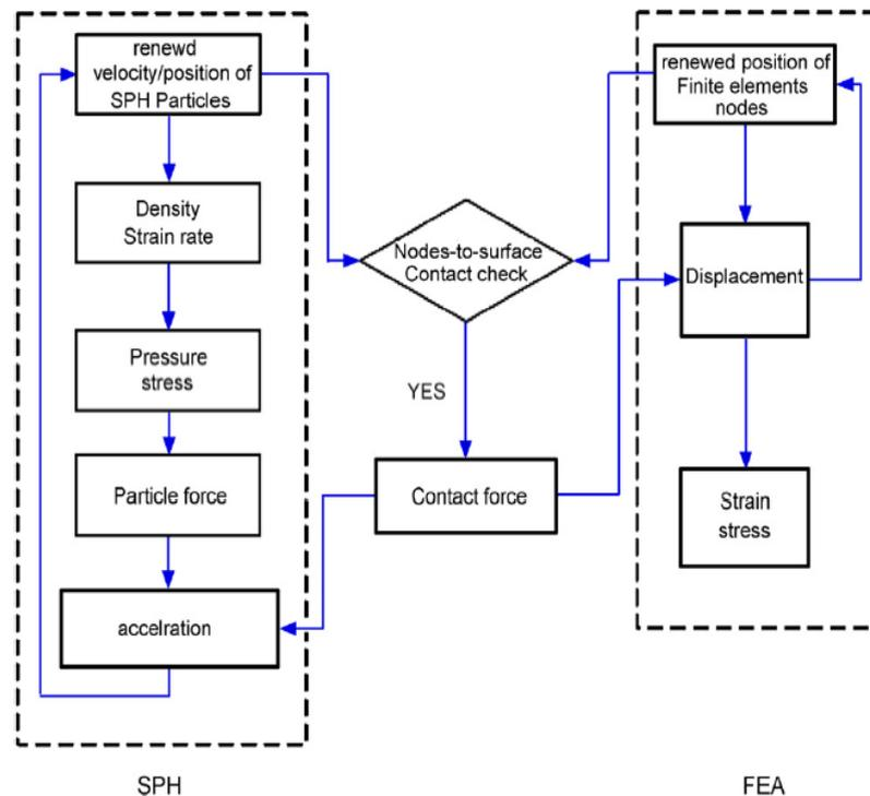
Fig. 2 SPH-FEM coupling technique [9]
