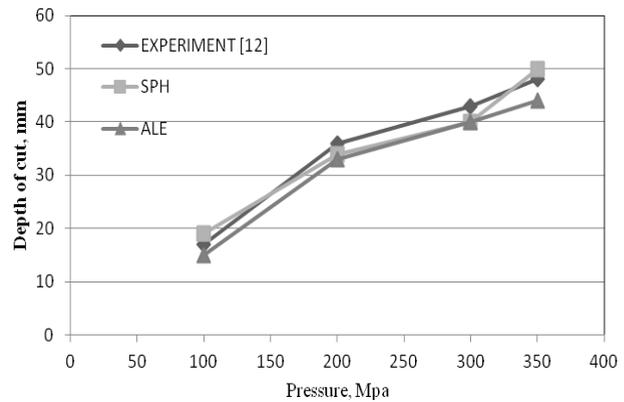
Fig. 8 Change of cutting depth under various pressures.
