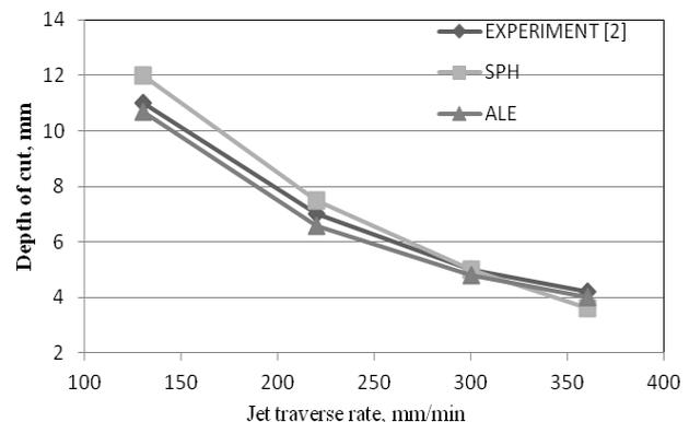
Fig. 9 Effect of jet transverse rate on the cutting depth
