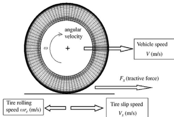
Fig. 2 Free body diagram of a single tire
