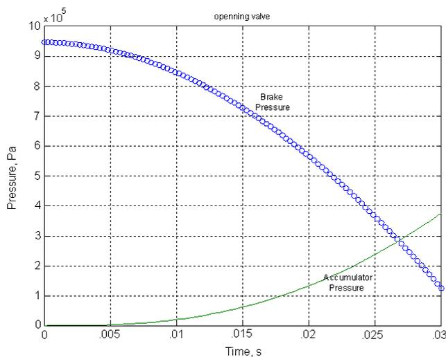
Fig. 10 The pressure variations of cylinder 2
