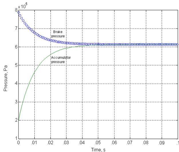
Fig. 9 The pressure variations of cylinder 1
