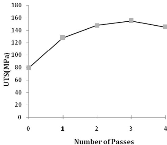
**Fig. 7** Ultimate tensile strength against number of passes
