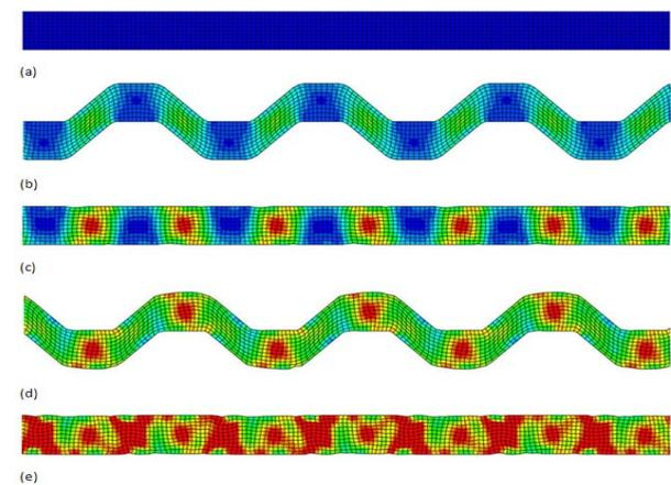
**Fig. 8** Equivalent plastic strain contours in different pressing steps (a) Initial (b) After first pressing step (c) After second pressing step (d) After third pressing step and (e) After fourth pressing step
