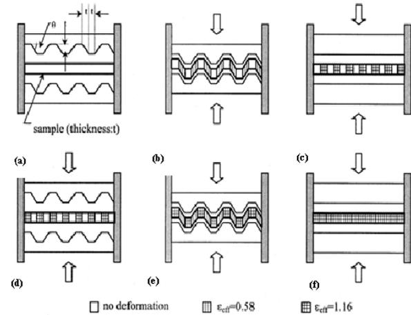
Fig. 1 Schematic of the sequences of the CGP [4]
