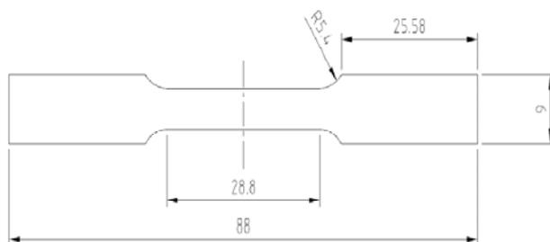
**Fig. 3** Dimensions of tensile test specimen (mm)
