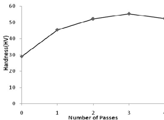
**Fig. 5** Mean of Vickers hardness variations with number of passes
