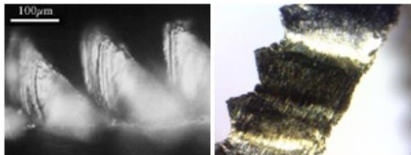
Fig. 4 Saw toothy chip taken by an optical micrographer
