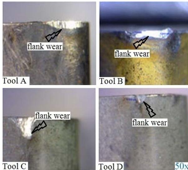
**Fig. 1** Flank wear region of alumina ceramic tools A, B, C, D
