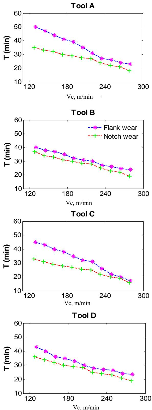
Fig. 5 Maximum allowable machining time vs. the cutting speed
