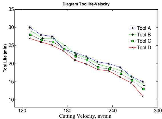
**Fig. 6** The tool life of the ceramic cutting tool at different cutting speeds
