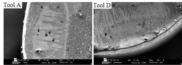
**Fig. 2** Crater wear region on the surface of the alumina ceramic tools A and D
