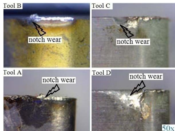
**Fig. 3** Notch wear region of the ceramic cutting tools A, B, C, D
