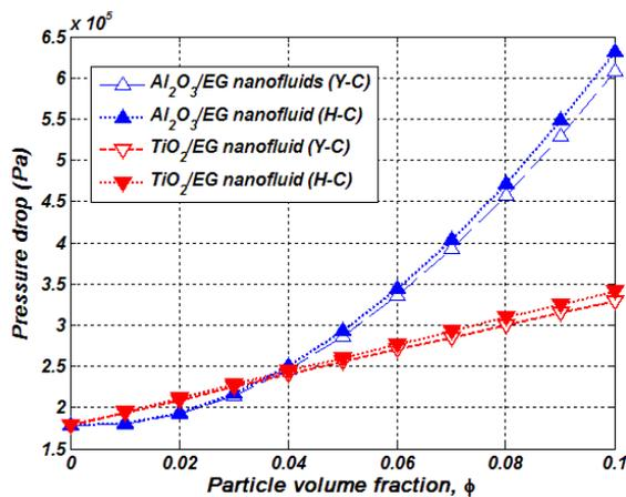
Fig. 9 Comparison of pressure drop for Al<sub>2</sub>O<sub>3</sub>/EG and TiO<sub>2</sub>/EG nanofluids
