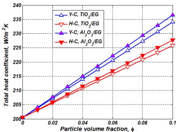
Fig. 4 Total heat transfer coefficient of Al<sub>2</sub>O<sub>3</sub>/EG and TiO<sub>2</sub>/EG nanofluids as coolants in a double-tube heat exchanger
