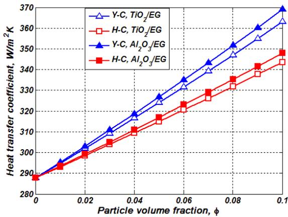
Fig. 3 Heat transfer coefficient of Al<sub>2</sub>O<sub>3</sub>/EG and TiO<sub>2</sub>/EG nanofluids as coolants in a double-tube heat exchanger
