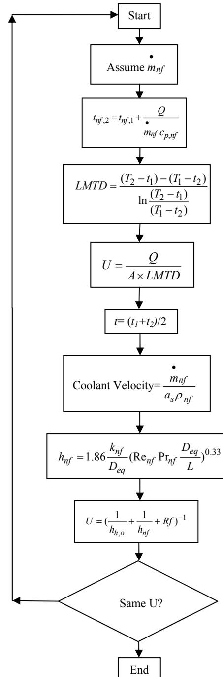
**Fig. 1** The flow diagram illustrates the calculating steps of the flow rate optimization of nanofluids as coolants in the double-tube heat exchanger
