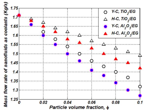
Fig. 7 Flow rate reduction of the coolant in a double-tube heat exchanger using Al<sub>2</sub>O<sub>3</sub>/EG and TiO<sub>2</sub>/EG nanofluids as coolants
