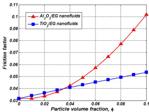
Fig. 8 Comparison of friction factor for Al<sub>2</sub>O<sub>3</sub>/EG and TiO<sub>2</sub>/EG nanofluids
