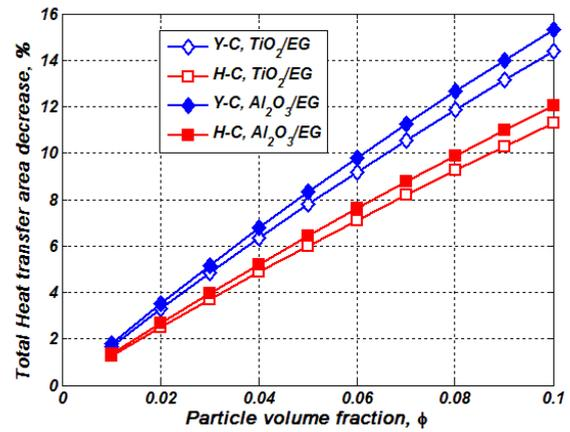
Fig. 6 Total heat transfer area reduction in a double-tube heat exchanger, using Al<sub>2</sub>O<sub>3</sub>/EG and TiO<sub>2</sub>/EG nanofluids as coolants
