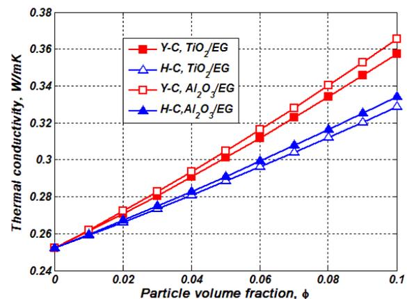
Fig. 2 Variation of thermal conductivity versus particle volume fraction for Al<sub>2</sub>O<sub>3</sub>/EG and TiO<sub>2</sub>/EG nanofluids
