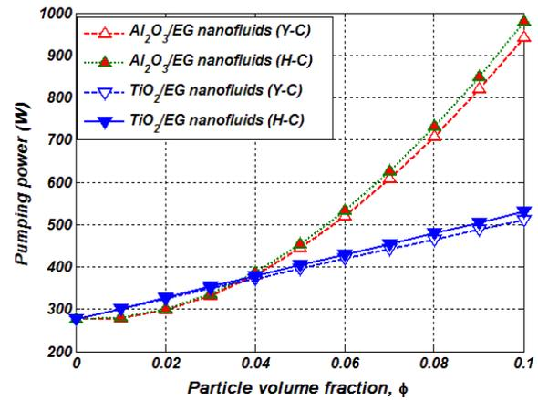
Fig. 10 Pumping power for Al<sub>2</sub>O<sub>3</sub>/EG and TiO<sub>2</sub>/EG nanofluids in a double-tube heat exchanger at different volume concentrations
