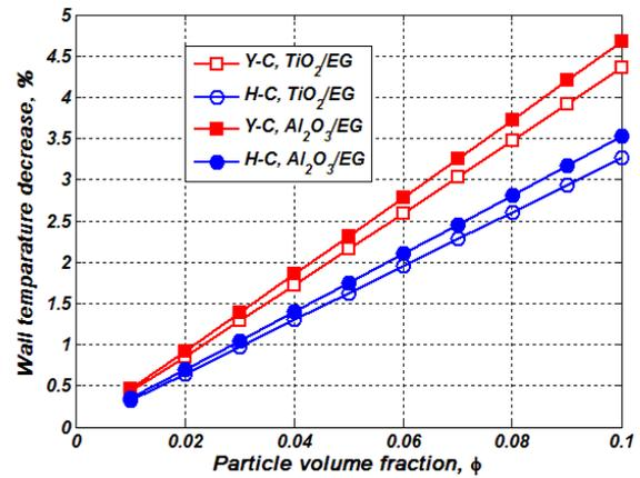
Fig. 5 Effect of nanoparticles volume fraction on wall temperature in a double-tube heat exchanger
