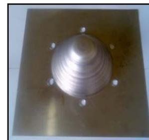
Fig. 6 Conically formed sheet
