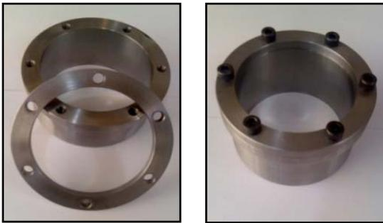
Fig. 1 Fixture including main base and ring piece
