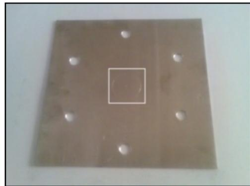
Fig. 9 Drawing of circle on the back and centre of the sheet
