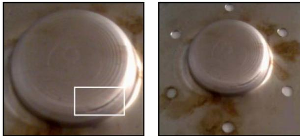
Fig. 10 Failure zone in the formed sheet by first strategy
