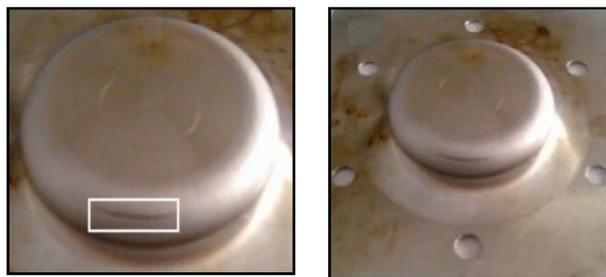
Fig. 11 Failure zone in the formed sheet by second strategy
