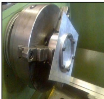
Fig. 4 Attaching the fixture to the chuck
