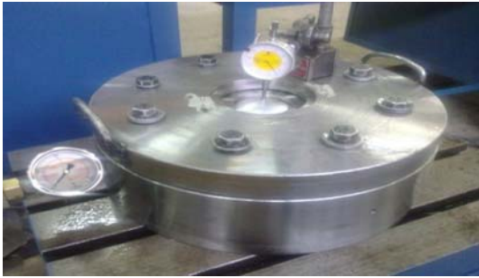
Fig. 2 Hydroforming bulge test apparatus
