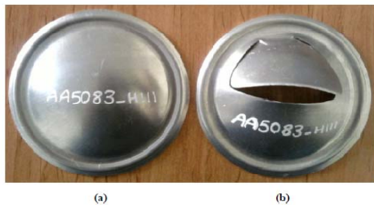
Fig. 9 Hydraulic bulge test samples (a) sample not burst and (b) sample burst
