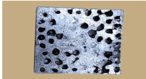
**Fig. 9** Porous casting at 950°C
