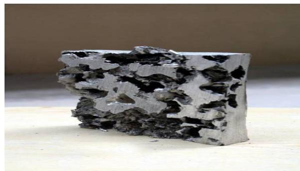
Fig. 5 Soaked Precursors at 850°C (using aluminum net)
