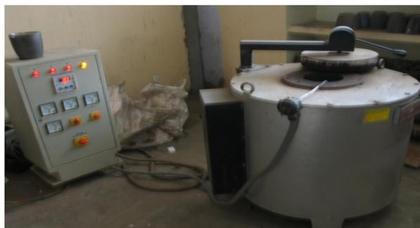
Fig. 2 Electrically heated crucible furnace
