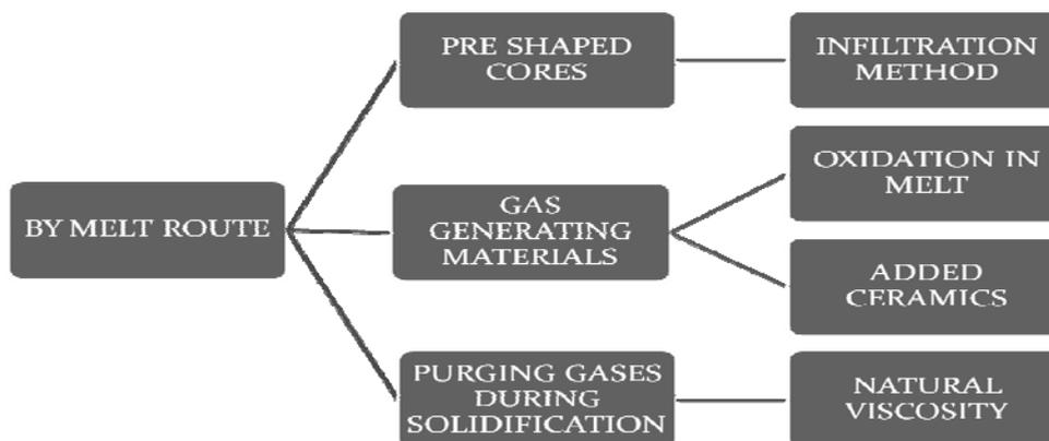
Fig. 1 Melt route methods for production of metal foams
