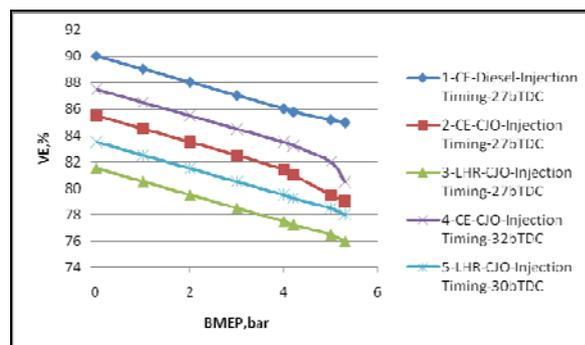
**Fig. 6** Variation of volumetric efficiency (VE) with brake mean effective pressure (BMEP) in conventional engine (CE) and low heat rejection (LHR) engine at recommended injection timing and optimized injection timings
