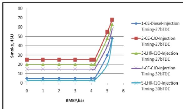
Fig. 7 Variation of smoke intensity in Hartridge Smoke Unit (HSU) with brake mean effective pressure (BMEP) in conventional engine (CE) and low heat rejection (LHR) engine at recommend injection timing and optimized injection timings
