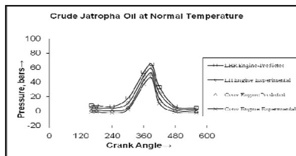
**Fig. 9** Comparison of typical pressure-crank angle data predicted from the multi-zone combustion model and the experimental values obtained from the special P- $\theta$  software package and TDC encoder for the case of conventional and LHR engines at the recommended injection timing and injection pressure
