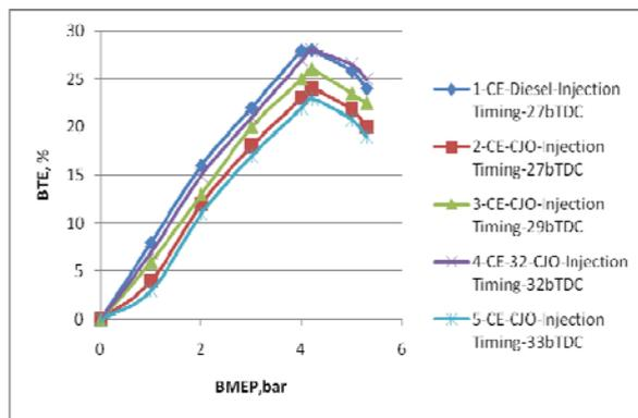
**Fig. 3** Variation of brake thermal efficiency (BTE) with brake mean effective pressure (BMEP) in conventional engine (CE) at different injection timings
