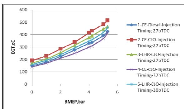
**Fig. 5** Variation of exhaust gas temperature (EGT) with brake mean effective pressure (BMEP) in conventional engine (CE) and low heat rejection (LHR) engine at recommended injection timing and optimized injection timings
