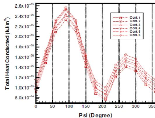
**Fig. 2** TCHG for different configurations in with respect to changes in wall orientation
