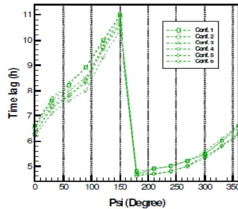
Fig. 4 TL for different configurations in with respect to changes in wall orientation
