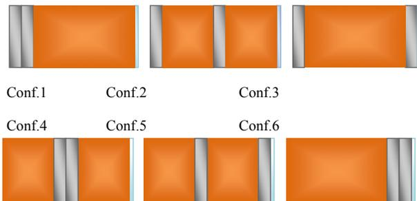
**Fig 1** Six possible wall configurations using two masonry material layers, two insulation layers and one gypsum layer
