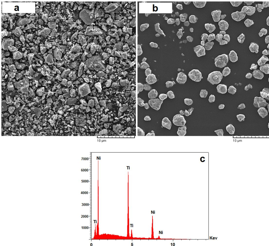
Fig. 4 SEM images of milled powders after: (a) 10h and (b) 40h milling, and (C) EDS spectrum of sample b
