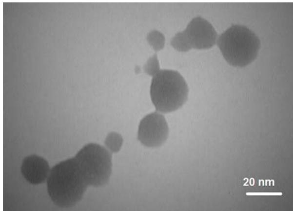
**Fig. 5** TEM images from of as-milled powders after 60h in two different magnifications
