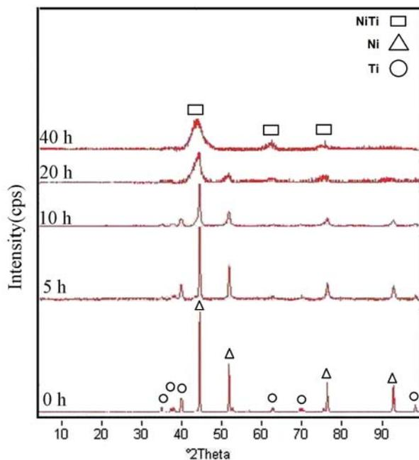
Fig. 2 XRD diffraction patterns of powders at several milling times
