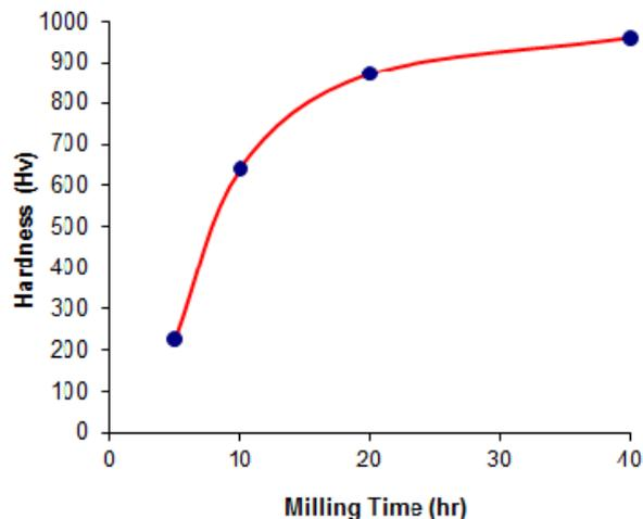
**Fig. 6** Micro hardness values of NiTi alloy as a function of milling time
