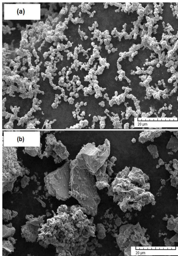
Fig. 1 SEM images of initial powders: (a) Ni and (b) Ti
