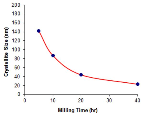
Fig. 3 Crystallite size of mixture powders at diffraction milling times
