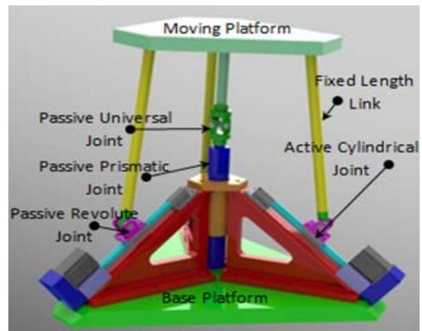
Fig. 1 CAD model of 3-CRS/PU parallel manipulator
