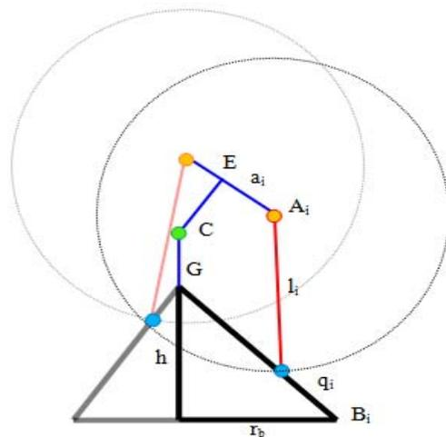
Fig. 3 Schematic configuration of 3-CRS kinematic
