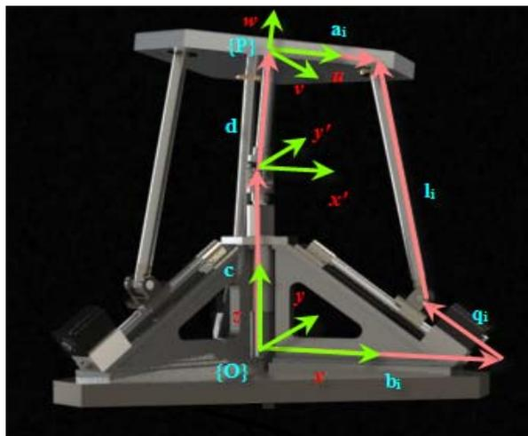
Fig. 2 Geometrical Model of 3-CRS/PU
