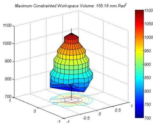
**Fig. 9** Optimal workspace for the case study mechanism
