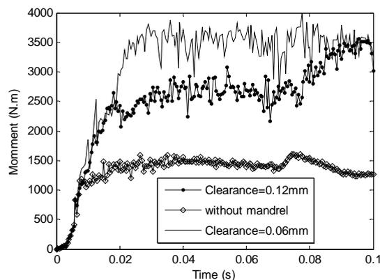
Fig. 7 Comparison between required torques for bending in three different models (model without mandrel, model with mandrel and 0.12mm clearance, model with mandrel and 0.06mm clearance)
