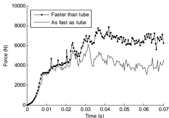
**Fig. 10** Comparison of the required force for displacing the pressure die between two models (model with moving pressure die in a speed equal to tube's speed and model with moving pressure die in a speed greater than tube's speed)
