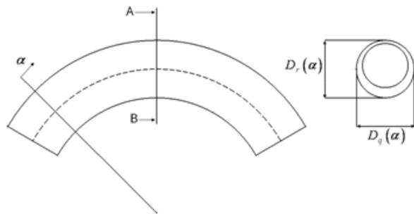
Fig. 8 Calculation of the flattening value
