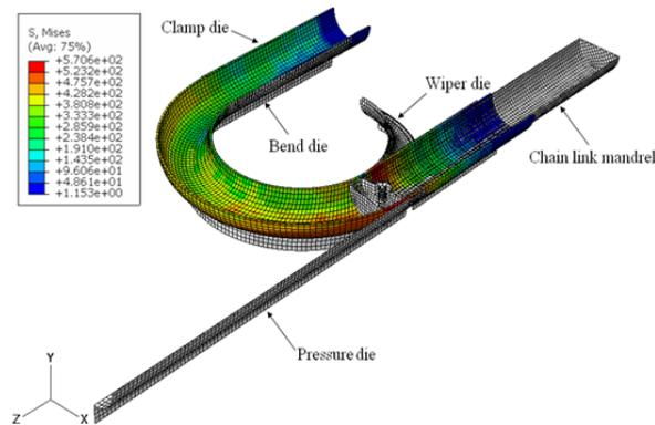
Fig. 2 Bending process modeling of tube with 38mm diameter, 79mm bend radius and 1.58mm thickness
