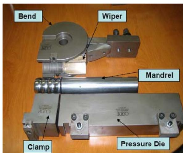
**Fig. 1** Major components in rotary draw bending technique
