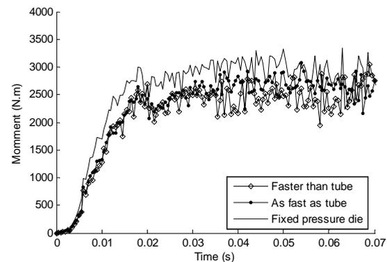
Fig. 9 Comparison of required bending moment between three different models (model with fixed pressure die, model with moving pressure die in a speed equal to tube's speed, model with moving pressure die in a speed greater than tube's speed)
