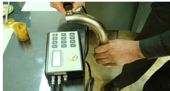
Fig. 4 Measuring the bent tube thickness by ultrasonic thickness measuring device
