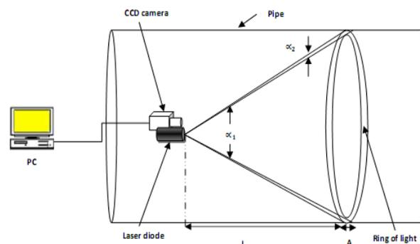
Fig. 1 Schematic view of the optical system
