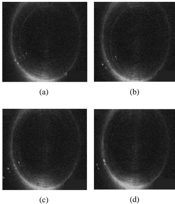
**Fig. 4** Light ring images: (a) 2mm diameter hole, (b) 3mm diameter hole, (c) 4mm diameter hole, (d) 5mm diameter hole
