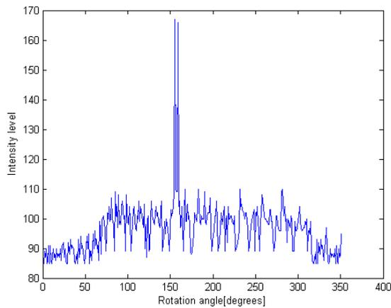
**Fig. 6** Intensity diagram for defective profile of 2mm hole diameter
