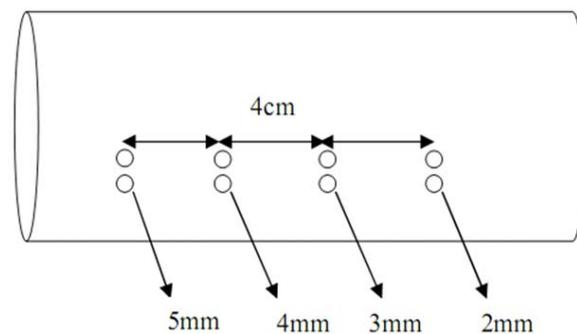
Fig. 3 Schematic of the test specimen with holes
