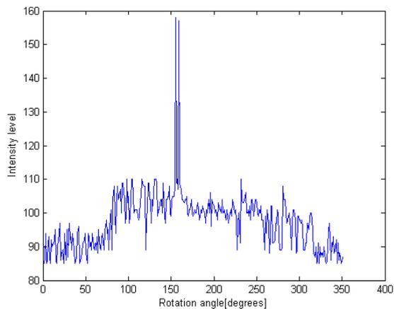
**Fig. 8** Intensity diagram for defective profile of 4mm hole diameter
