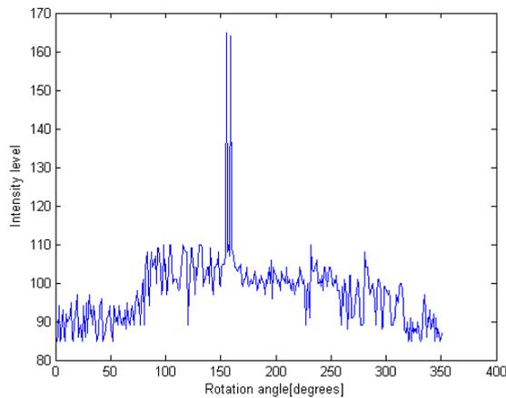
**Fig. 7** Intensity diagram for defective profile of 3mm hole diameter
