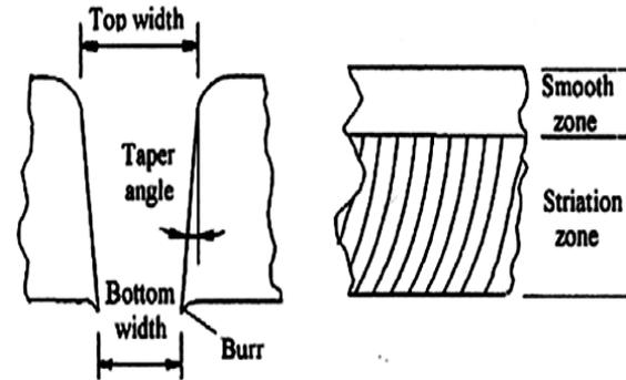
Fig. 2 Schematic and definition of kerf geometry [6]
