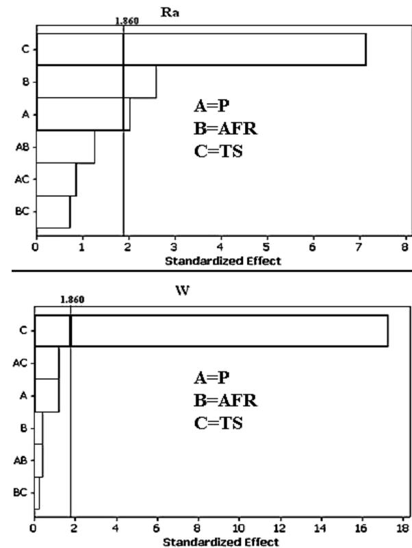
Fig. 8 Standardized effect of the parameters on the Kerf width and surface roughness
