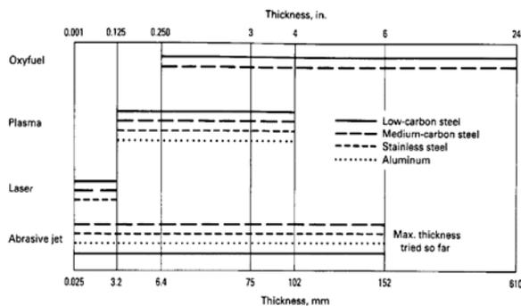
Fig. 1 Comparison of applying different cutting methods for various work piece thicknesses [2]
