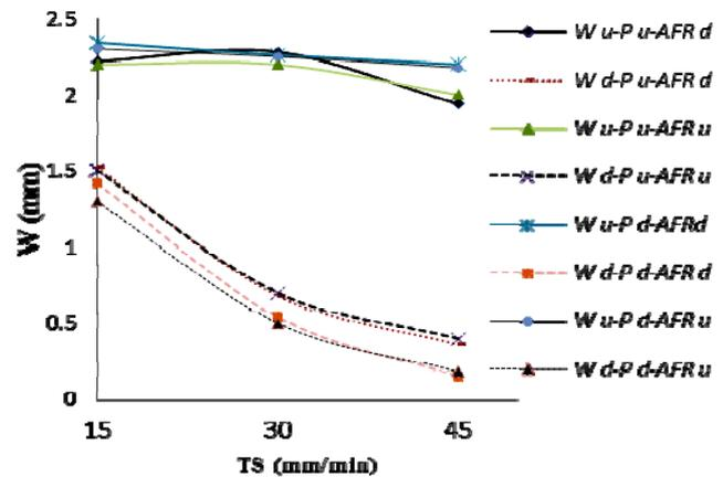
**Fig. 4** Diagram of kerf width in the upper and lower sections relation the TS ( $P_u=3800$  bar &  $P_d=3500$  bar and  $AFR_u=400$  g/min &  $AFR_d=300$  g/min)
