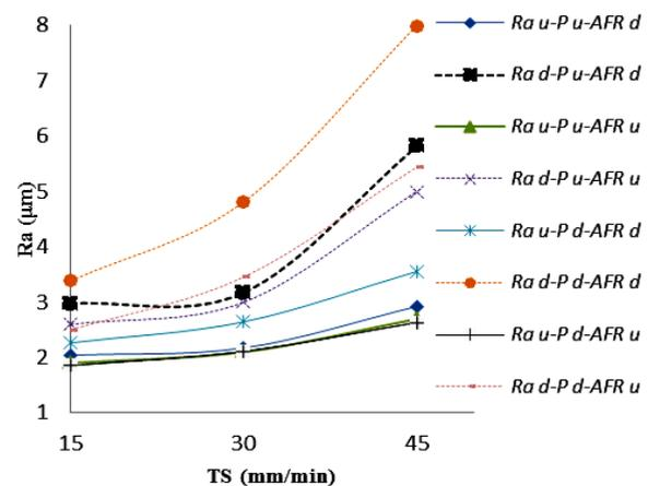
**Fig. 5** Diagram of the surface roughness to the TS ( $P_u=3800$  bar &  $P_d=3500$  bar and  $AFR_u=400$  g/min &  $AFR_d=300$  g/min)
