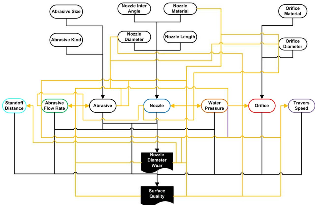
Fig. 3 Relation between different parameters in AWJ machining process
