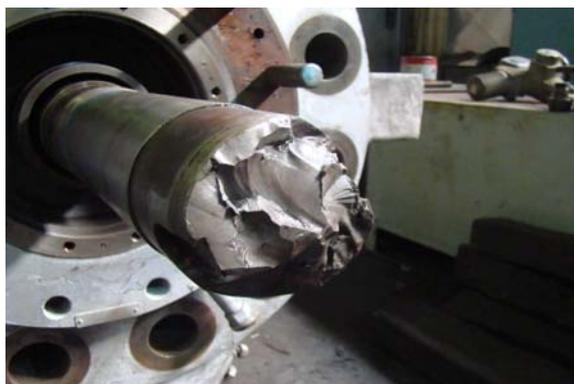
Fig. 3 Shaft failure location of feedwater pump
