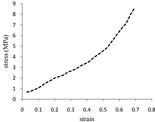
**Fig. 4** Experimental compression stress–strain curve for natural rubber
