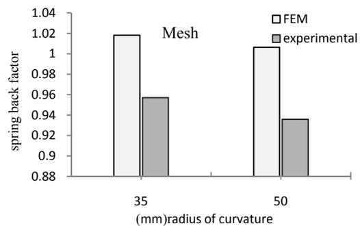
Fig. 13 FE results compared to simulation results
