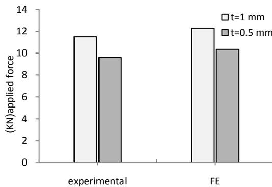
Fig. 7 Comparison of applied force for shaping the blank with variable thickness (radius of curvature 35 mm)
