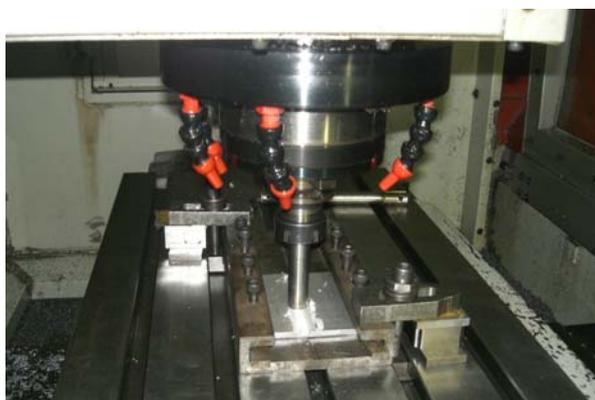
Fig. 5 FSW Processing set-up
