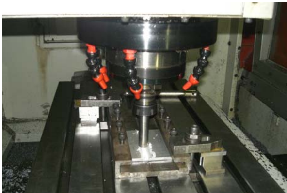
Fig. 5 FSW Processing set-up
