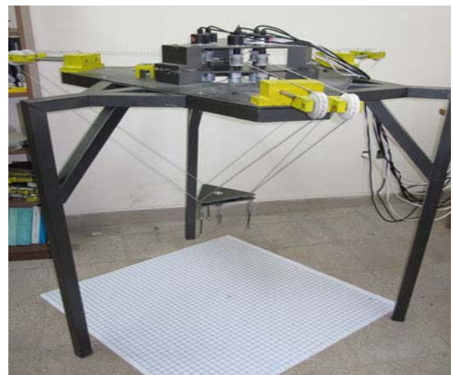
Fig. 5 Scheme of the designed IUST cable robot
