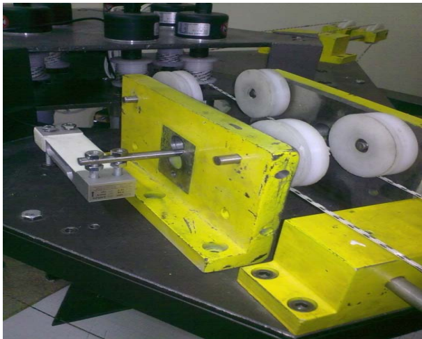
Fig. 2 Loadcell used as the tension sensing device
