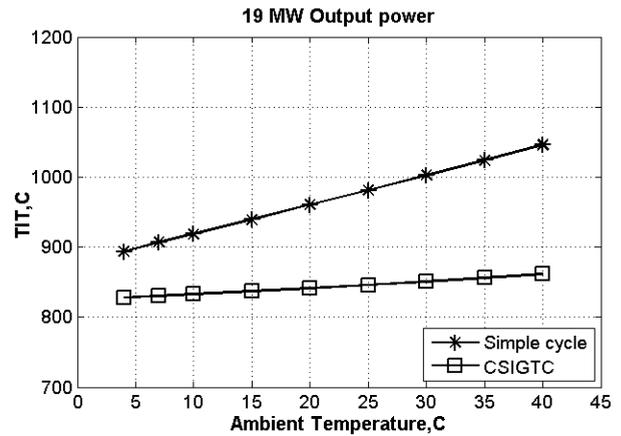
Fig. 9 The variation of TIT against ambient temperature
