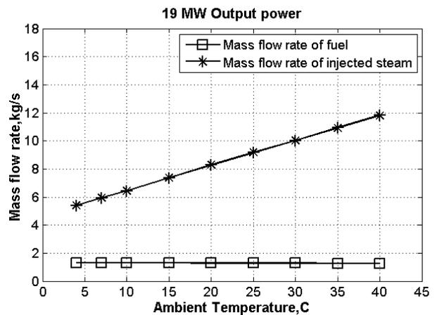
Fig. 10 The variation of fuel and steam mass flow against ambient temperature
