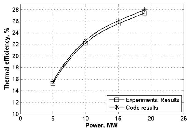
Fig. 4 Comparison of the model and experimental results [20] of the GE-F5 simple gas turbine cycle
