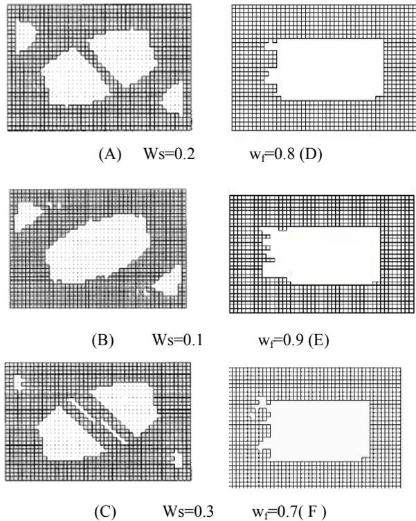
Fig. 3 Optimal designs of rectangular plate for different weighting criteria of stiffness and natural frequency; material removed, 30%. (A)-(C) [10], (D) – (F) BCO Method
