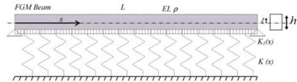
**Fig. 1** FG beam supported on two-parameter elastic foundation
