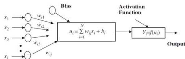
Fig. 2 Basic elements of an artificial neuron
