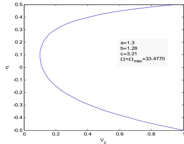
**Fig. 11** Optimized material profile for maximum natural frequency
