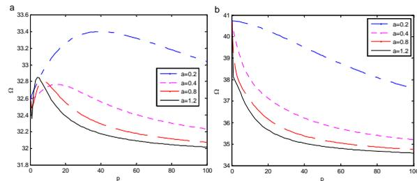
**Fig. 7** Variation of the natural frequency parameter vs. the power-law exponent  $p$  for various values of the parameter  $a$  and different boundary conditions ( $0.2 \leq a \leq 1.2, b = 0.2, c = 2$ )
