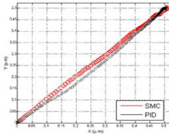
**Fig. 7** Comparison control motion of nano-particle from the (0,0) point to (0.5 $\mu$ m,0.5 $\mu$ m) position during pushing to validate the presented sliding controller
