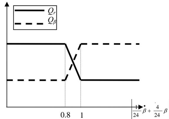
Fig. 3 Adaptation of weighting coefficients based on phase plane notion
