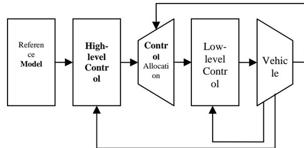
Fig. 1 Integrated optimal control scheme
