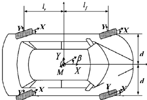
Fig. 4 Vehicle plane motion parameters
