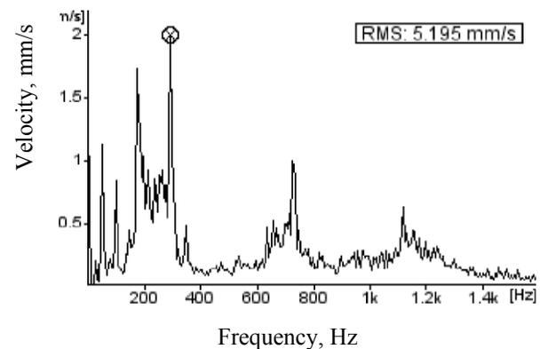
Fig. 1 Velocity response of pump before attaching TVA
