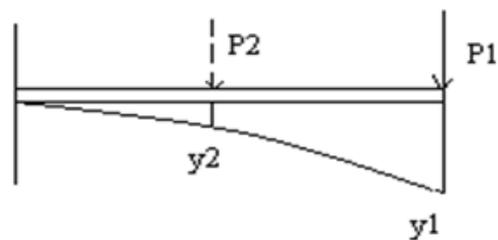
Fig. 3 Cantilever beam with assumed deflection
