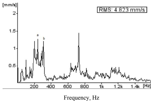
Fig. 8 Velocity response of Pump after attaching TVA, a): 243Hz, b): 312 Hz
