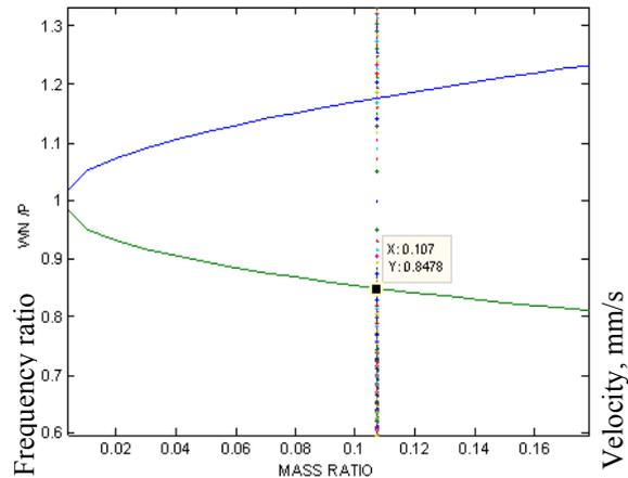
Fig. 6 Two new natural frequencies in relation to mass ratio of the TVA
