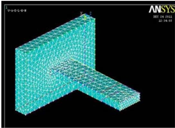
Fig. 4 FE Meshed model of TVA
