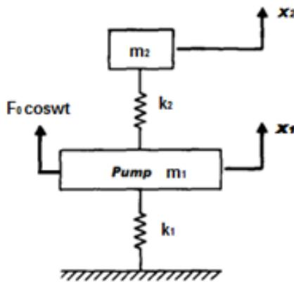
Fig. 5 Pump system and TVA model
