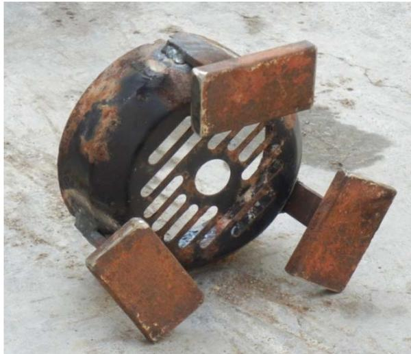
Fig. 2 TVA welded to the fan cover
