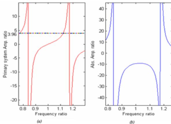
Fig. 7 Amplitude ratio to frequency ratio of primary system (a), Absorber system (b)
