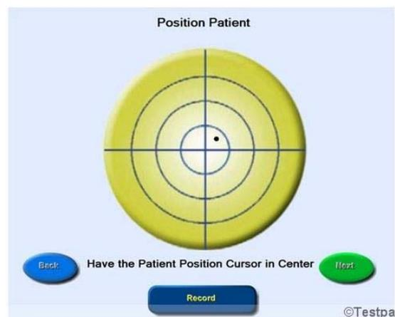
**Fig. 6** The Centering Process form. The person is engaged to position feet such that the black point of COP on the circle target intersects the origin. Then pressing Record stops the process and coordinates of the feet are imported by the operator. This process is called Centering
