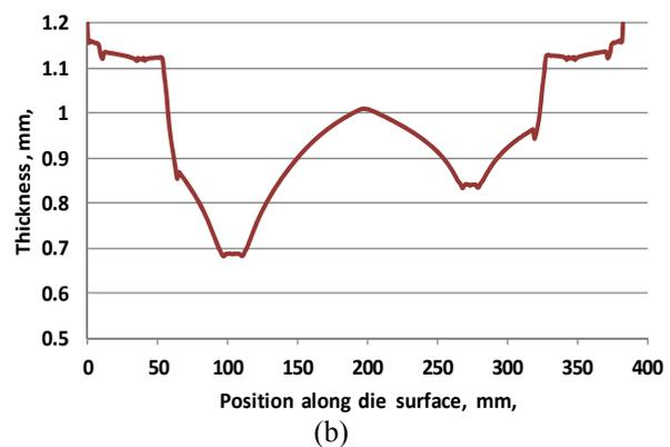
**Fig. 5** a) FE-predicted thickness profile at the mid-section of the formed panel with  $\mu=0.5$  (blue) [23], and compared with that obtained experimentally (black) using graphite as a lubricant, b) FE-predicted thickness profile (red) obtained in this study with  $\mu=0.5$
