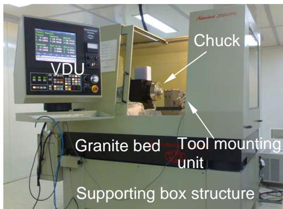
Fig. 1 Diamond Turning Machine
