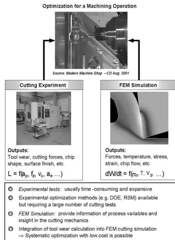
**Fig. 3** Comparison between experimental testing and FEM simulation for machining analysis
