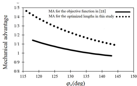
Fig. 10 Variation of the mechanical advantage in the penetration zone
