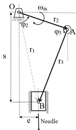
Fig. 1 The slider crank mechanism
