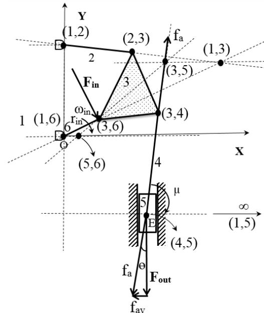
Fig. 3 The instant centers of the mechanism
