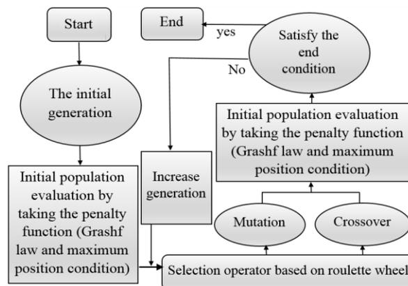
Fig. 4 Genetic Algorithm flowchart
