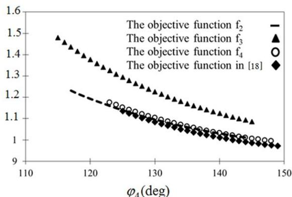
Fig. 12 Variation of the mechanical advantage in the penetration zone
