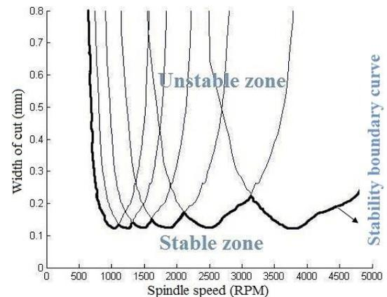
**Fig. 6** Stability lobe of boring process
