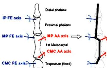
Fig. 1 Link model of the thumb [15]
