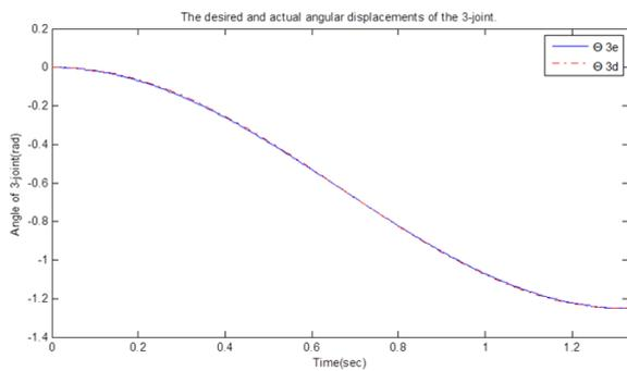
Fig. 22 Desired and actual angular displacements of joint 3
