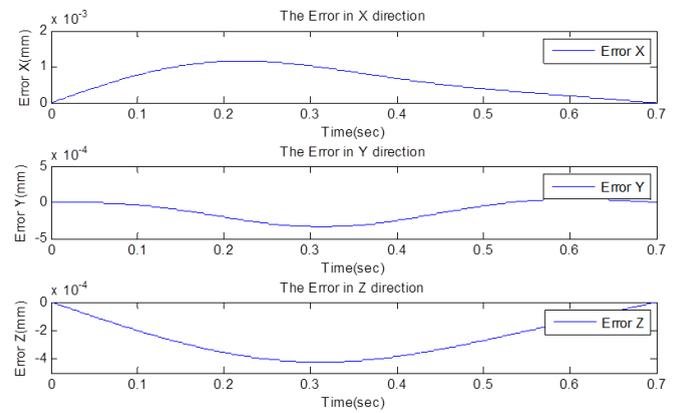
Fig. 12 Tracking error of Exoskeleton in Desecration coordinate
