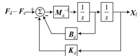
Fig. 5 Structure diagram of the impedance control compensator
