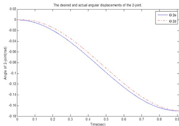
Fig. 14 Desired and actual angular displacements of joint 2
