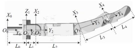
Fig. 2 Cartesian coordinate system in the thumb model
