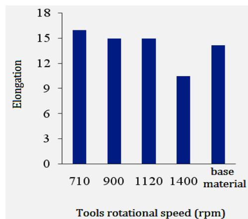
Fig. 9 Elongation of welded samples in different tools rotational speeds (traverse speed = 180 mm/min).
