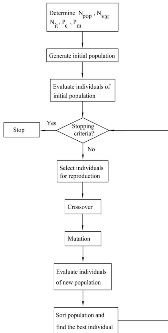
Fig. 4 A flowchart for the genetic algorithm method
