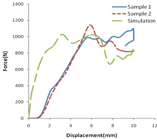
Fig. 12 Predicted and experimental force–displacement curves of 22 mm panels under quasi-dynamic impact
