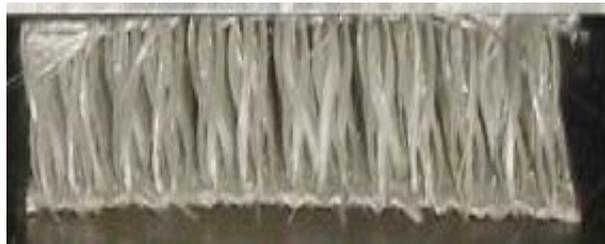
**Fig. 1** Cross section of 3D woven sandwich composites
