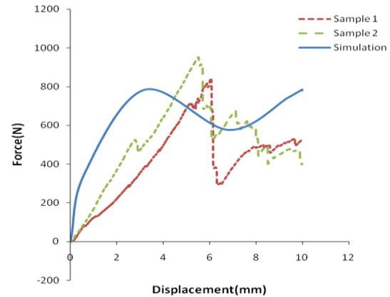
**Fig. 10** Predicted and experimental force–displacement curves of 22 mm panels under quasi-static indentation
