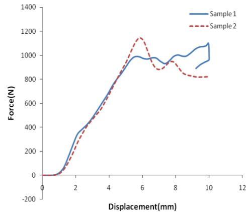
Fig. 5 Force-displacement curve in the quasi-dynamic for two similar tests
