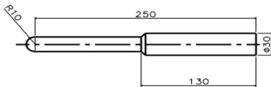
Fig. 3 Schematic of the mandrel used for experiments
