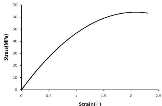
**Fig. 8** Tensile stress-strain behavior of ML-506 resin
