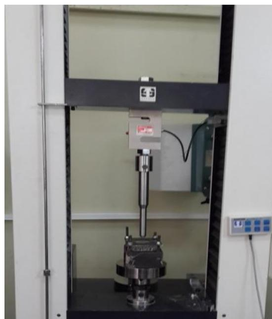
**Fig. 2** Universal testing machine used for experiments
