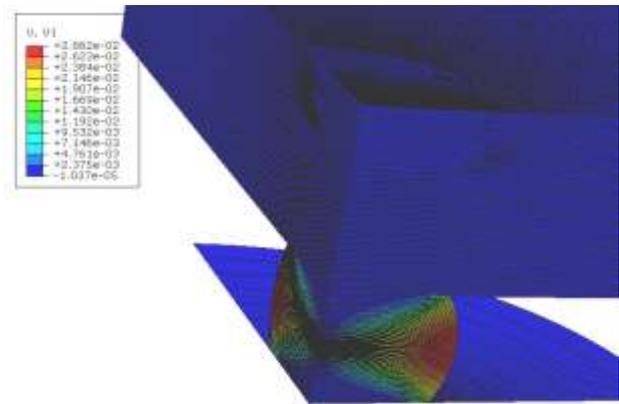
Fig. 25 The deformation contour in direction of the rivet radius
