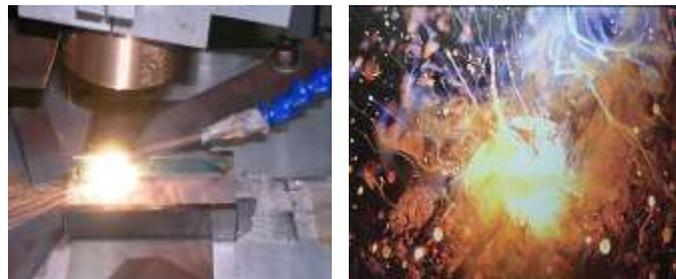
**Fig. 13** Laser cladding of preplaced powder
