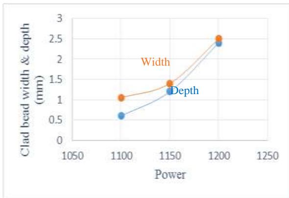
**Fig. 10** The relationship of laser power to depth and width
