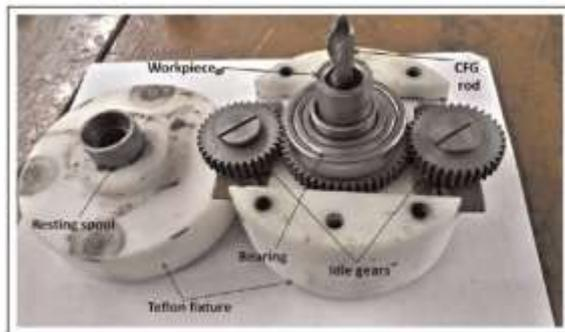
**Fig. 7** Elements of the rotating attachment used in the CFAAFM set-up [35]
