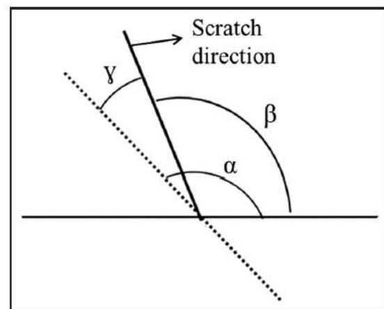
**Fig. 8** Active abrasive grain scratch at an angle  $\beta$  [51]
