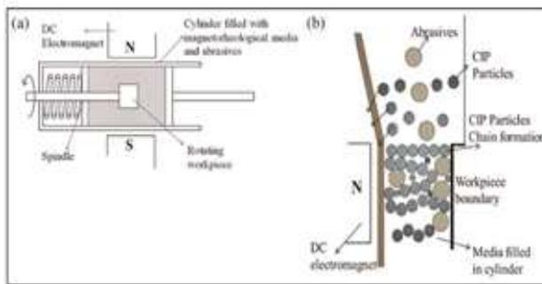
**Fig. 6** (a) Schematic of magnetorheological abrasive honing (b) Rearrangement of CIPs and abrasives during the process [44]
