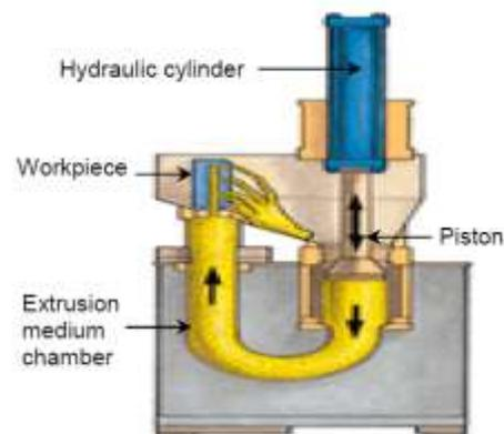
Fig. 2 Unidirectional AFM process [2]
