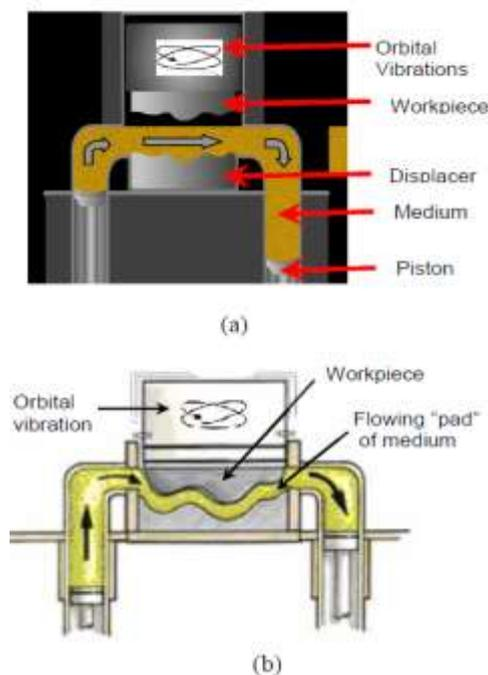
**Fig. 3** Orbital AFM (a) Before start of finishing, (b) While finishing [3]
