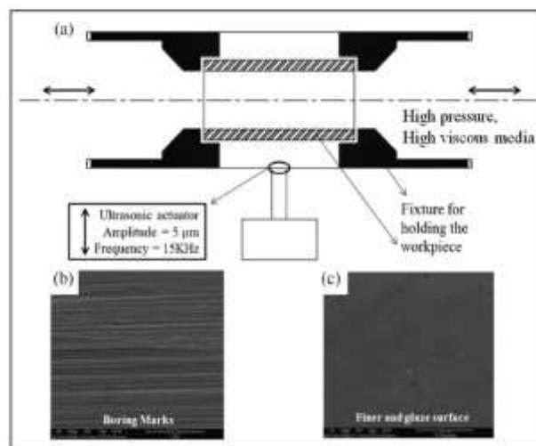
Fig. 10 (a) Schematic of UAAFAM, comparative study of the surfaces; (b) before UAAFAM and after UAAFAM [45]
