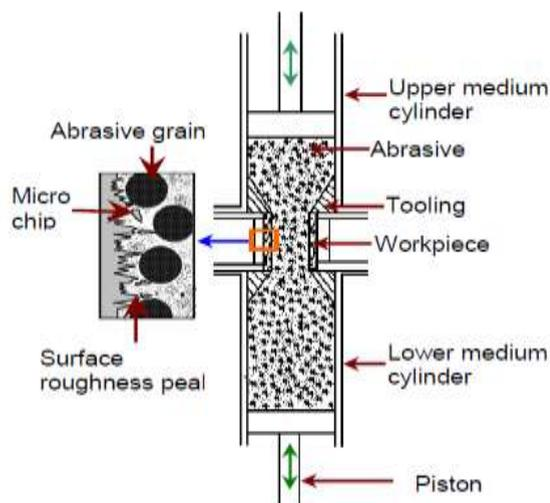
Fig. 1 Two way AFM process [4]
