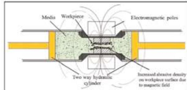
Fig. 5 Schematic of MAAFM set-up [35]
