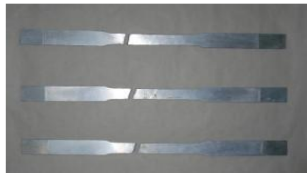
Fig. 4 The samples after tensile test experimental test
