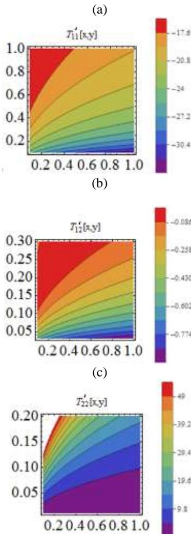
Fig. 8 Dimensionless stress components on a plate in the  $x$ - $y$  plane for  $C = -0.5$  for  $Wi = 10$
