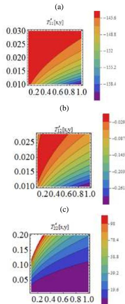
Fig. 7 Dimensionless stress components on a plate in the  $x$ - $y$  plane for  $C = 0$  for  $Wi = 100$
