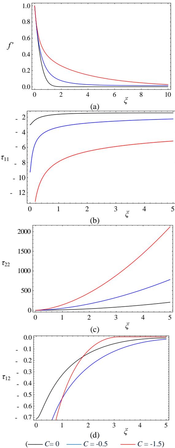
Fig. 2 Velocity and stress profiles for several values of pressure gradient constant,  $C$
