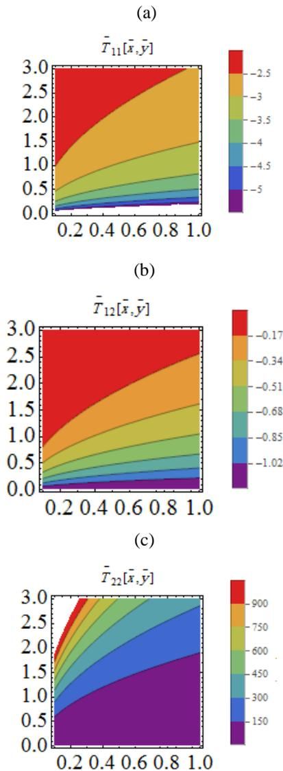
Fig.4 Scaled stress components in x-y plane for C = -0.5
