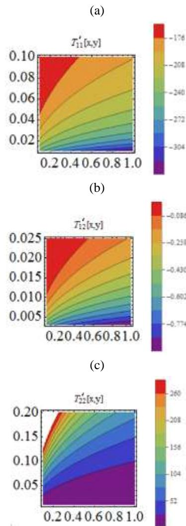
Fig. 9 Dimensionless stress components on a plate in the  $x$ - $y$  plane for  $C = -0.5$  for  $Wi = 100$
