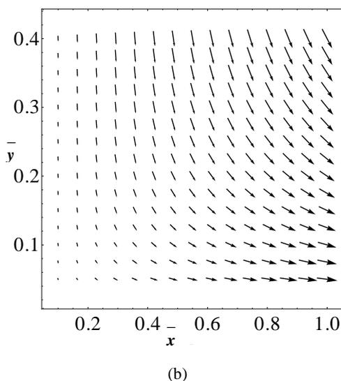
**Fig. 10** Development of scaled (a) Stream lines and (b) Velocity vector field for viscoelastic boundary layer ( $C=0$ )
