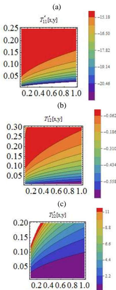
Fig. 6 Dimensionless stress components on a plate in the  $x$ - $y$  plane for  $C = 0$  for  $Wi = 10$
