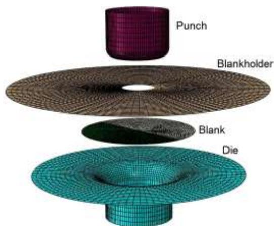
Fig. 1 Tools used in finite element simulations
