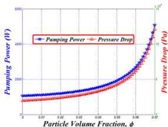
Fig. 5 Influence of  $\gamma$ -Al<sub>2</sub>O<sub>3</sub> volume fraction on the pumping power and pressure drop
