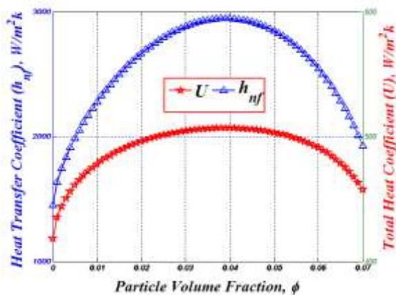
Fig. 3 Heat transfer coefficient and total heat transfer coefficient for  $\gamma$ -Al<sub>2</sub>O<sub>3</sub>/n-decane nanofluid at various concentrations
