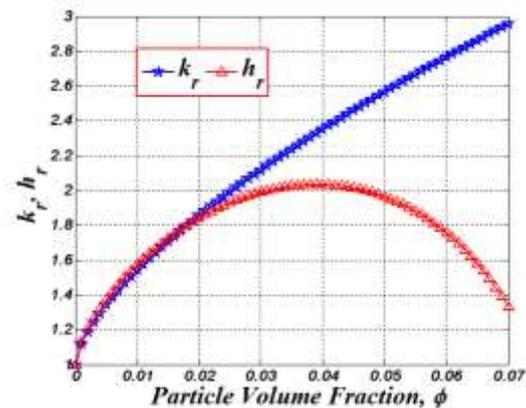
Fig. 2 Comparison between  $k_r$  and  $h_r$  for  $\gamma$ - $Al_2O_3$ /n-decane nanofluid flowing through tubes
