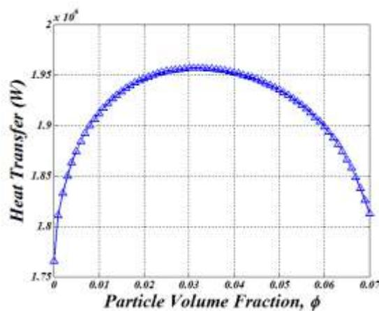
Fig. 4 Heat transfer rate for nanofluid at different particle concentration level
