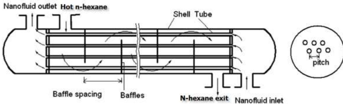
Fig. 1 Shell and tube heat exchanger configuration
