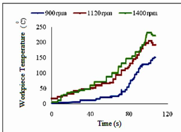
**Fig. 5** Effect of tool rotational speed on temperature distribution in workpiece (feed rate = 280 mm/min)
