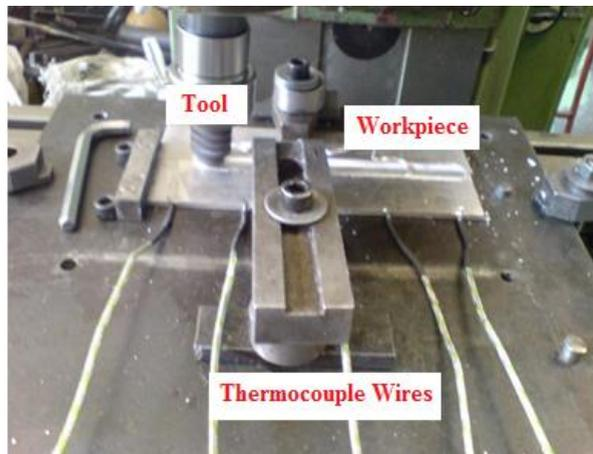
Fig. 1 The Welding machine used in this research with attached thermocouples on workpiece
