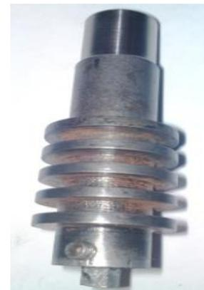
Fig. 2 The FSW tool used in this study
