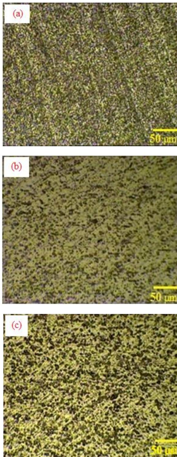
**Fig. 7** Microstructure of stir zone in 280 mm/min feed rate and different tool rotational speed, (a) 900 rpm, (b) 1120 rpm, (c) 1400 rpm
