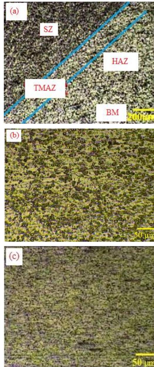
**Fig. 6** (a) Cross section view of weld obtained by friction stir welding and different regions around weld area, (b) base material microstructure, (c) nugget zone microstructure
