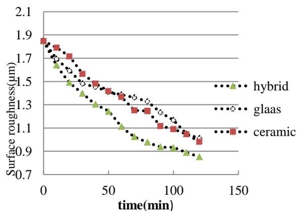
Fig. 5 The changes of surface roughness per time
