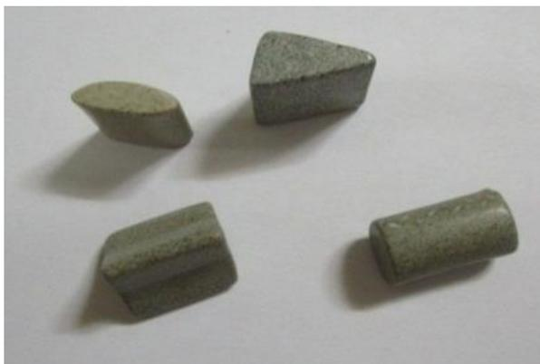
Fig. 3 The Abrasive ceramic particles.
