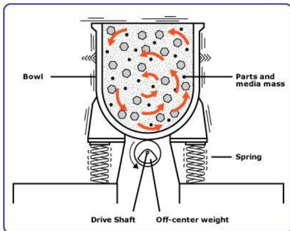
Fig. 2 The Schematics of the bowl-type vibratory finisher
