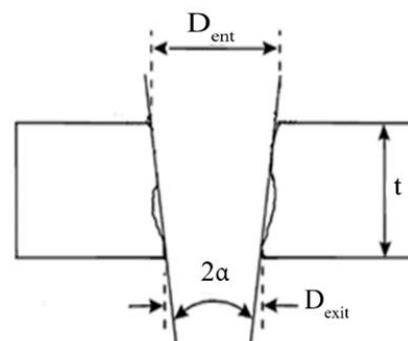
Fig. 1 The geometrical features of cross-section of the hole [15]
