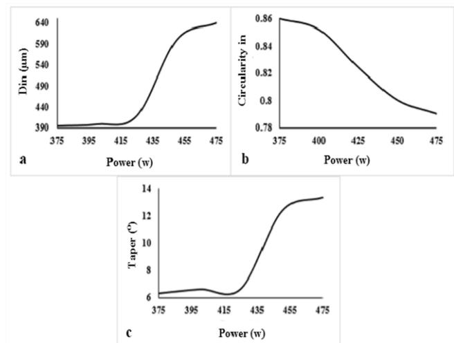
**Fig. 6** The Influences of the laser power on hole geometry features
