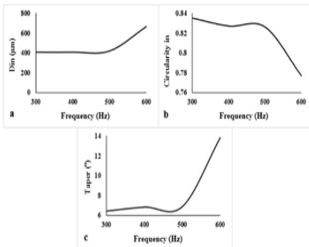
**Fig. 5** The Influences of laser pulse frequency on hole geometry features
