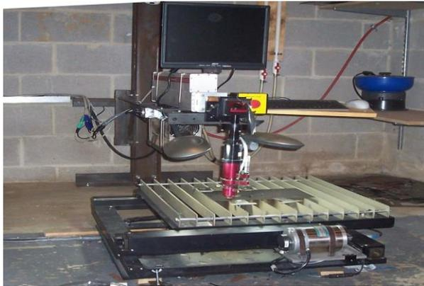
Fig. 4 The CNC CO<sub>2</sub> laser cutting
