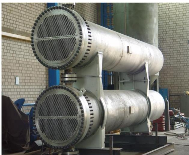
**Fig. 2** Perforated plates used in heat exchanges
