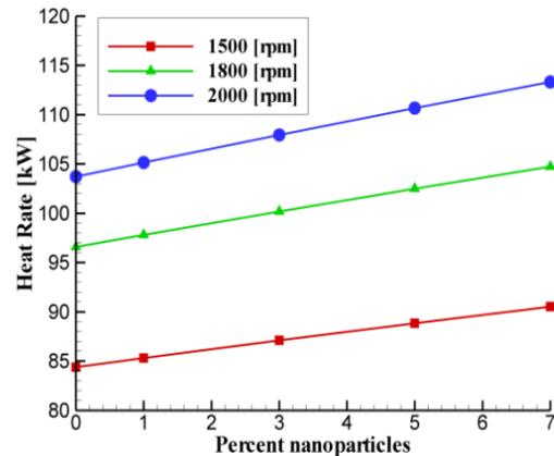
**Fig. 1** The Heat transfer rate for different volumetric densities of aluminum-oxide nanoparticle in base fluid at different fan speeds
