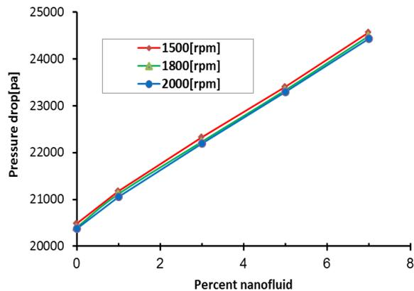
Fig. 2 The coolant pressure drop inside the radiator for different volumetric densities of aluminum-oxide
