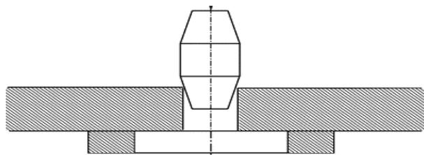
Fig. 1 Schematic of cold expansion process [2]
