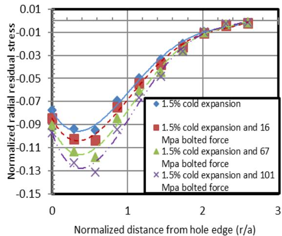
**Fig. 10** Radial residual stress field distribution in cross section and changes after closing bolts by three different pressure forces in mandrel entrance plate
