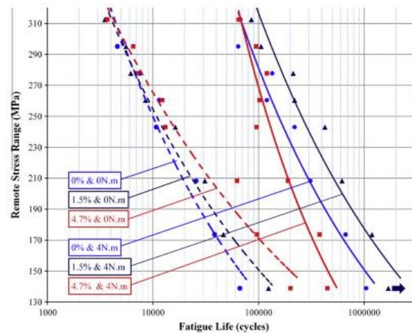
Fig. 12 S-N data obtained from fatigue tests [8]
