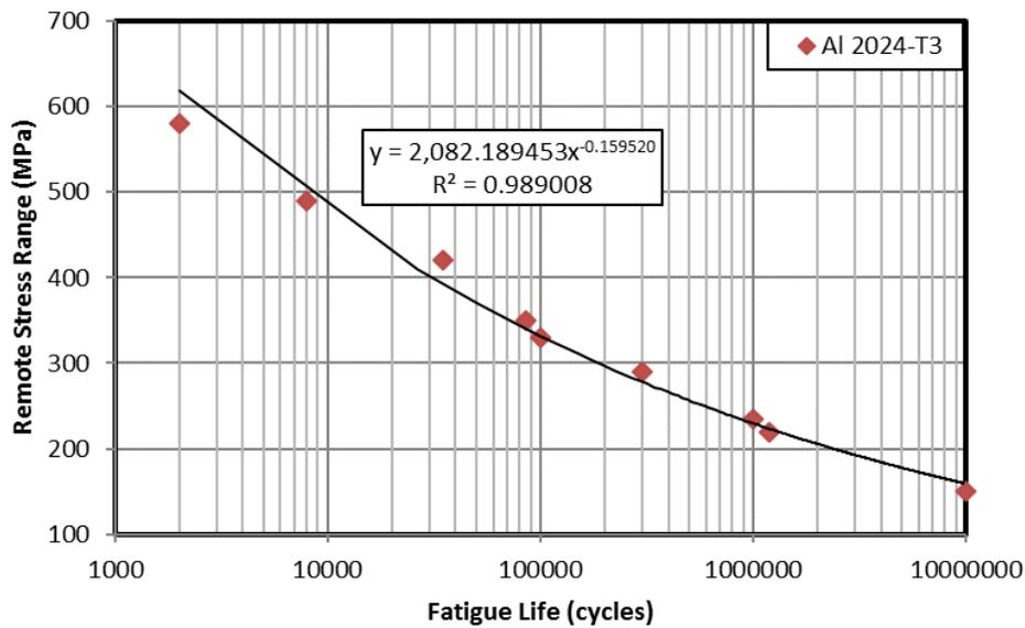
Fig. 13 The S-N diagram for Al 2024-T3
